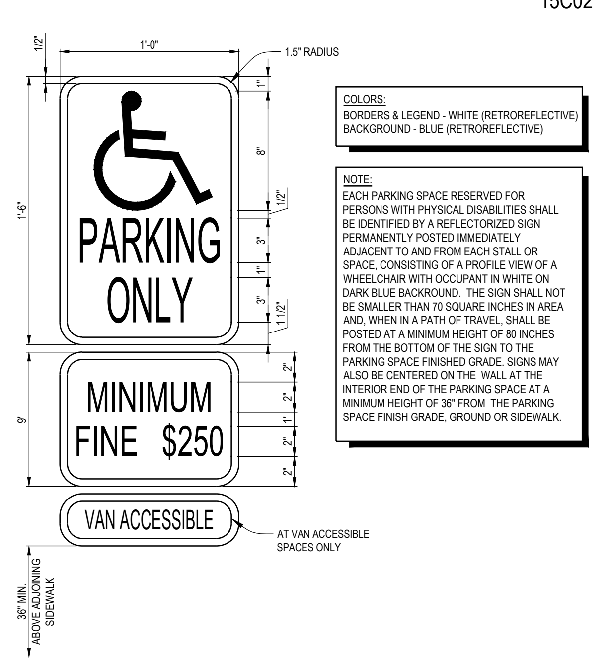
5 HANDICAP PARKING SIGNAGE (WALL MOUNTED) NO SCALE
